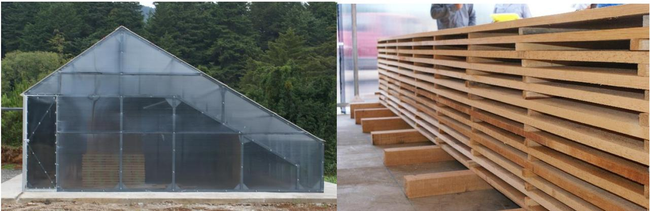
**Figure 3.** Solar greenhouse dryer for wood.
