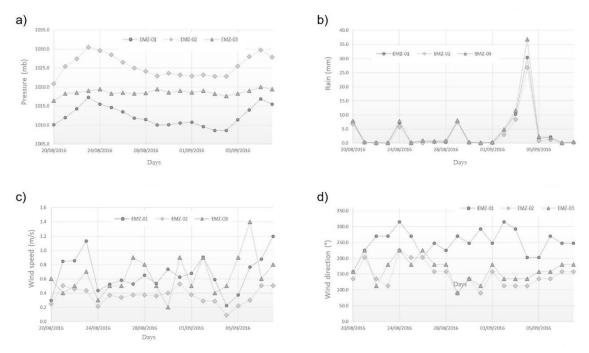
**Figure 8.** Data from the three stations of a) Pressure, b) Precipitation, c) Wind speed, and d) Wind direction.
