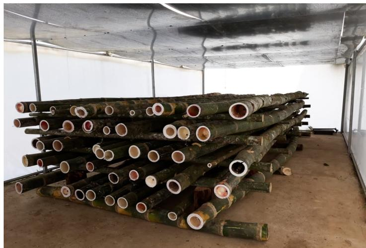
**Figure 2.** Stacking of *Guadua aculeata* Rupr. ex E. Fourn. culms inside the solar dryer.
