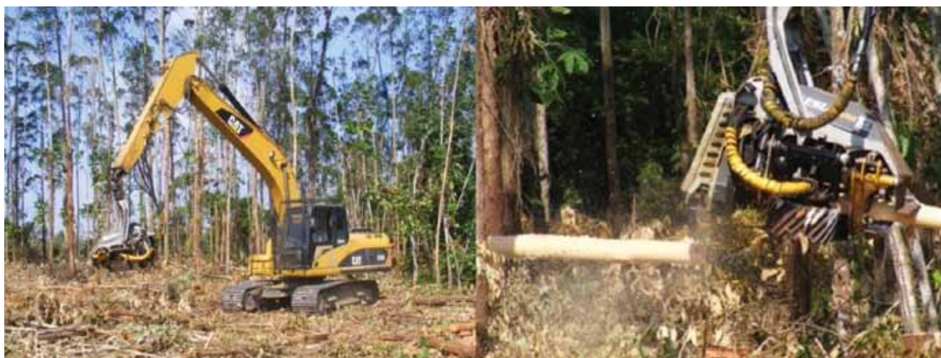
Figura 1. Cosechadora forestal, cabezal Kesla adaptado a la excavadora Caterpillar, Huimanguillo, Tabasco. Figure 1. Forest harvester, Kesla harvester head adapted to Caterpillar excavator, Huimanguillo, Tabasco.
